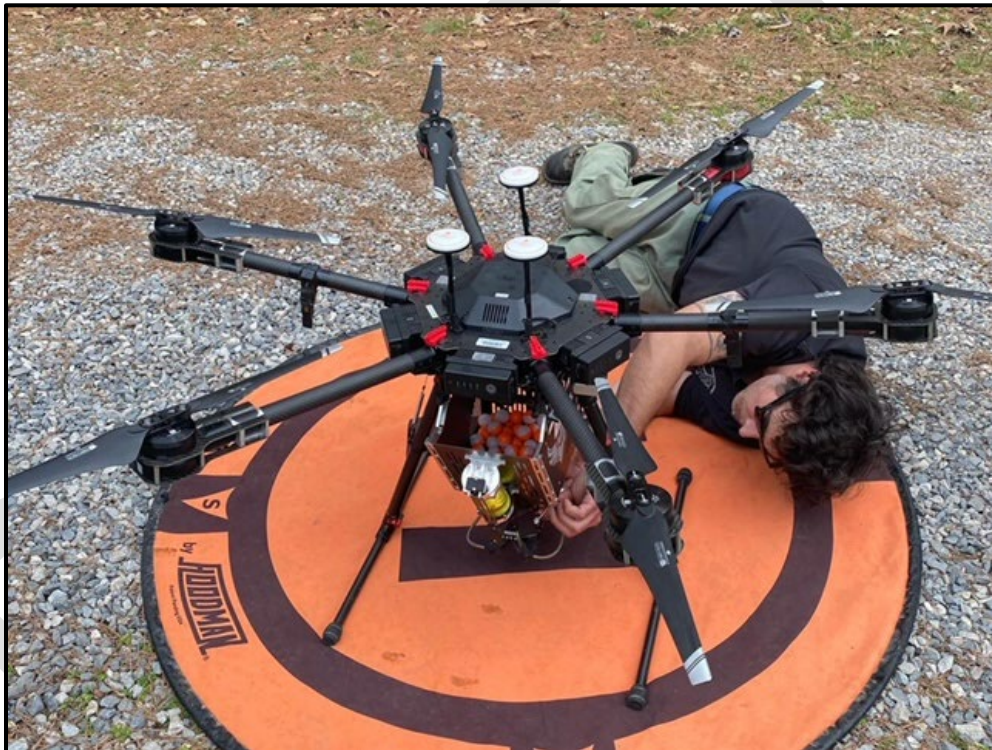
A drone used for aerial ignition of prescribed fire units. Using drones to ignite interior ridges reduces exposure to firefighters and allows burn bosses additional control over fire timing and intensity of prescribed fire.
